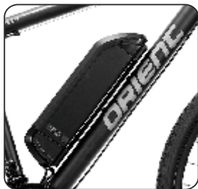
CENTRAL FRAME BATTERY Phylion 36V 10,4Ah
