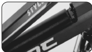
FRAME INTERGRADED BATTERY Phylion 36V 11,6Ah
